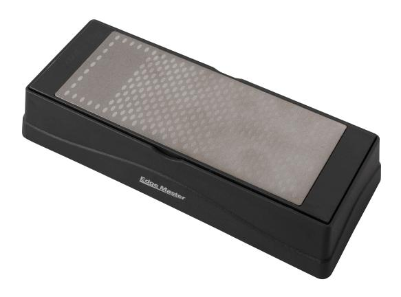
The Two-Sided Diamond Sharpening Stone from Edge Master features two sides, one coarse 360 grit side for rough work and one fine 600 grit side for fine work and will sharpen knives up to five times faster than using an oil stone or a whetstone. Industrial monocrystalline diamonds are electroplated onto a steel base and the super flat surface guarantees even contact with knives and tools.
